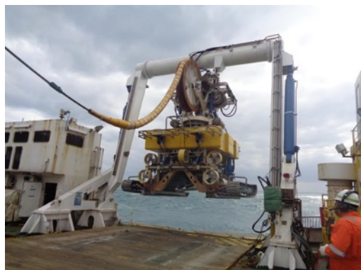
Deploying Sealion III during a telecom fibre optic cable repair operation (2020)
